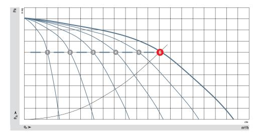
The following applies when operating several fans in parallel: the sum of the air flows from the individual fans equals the total air flow desired.
